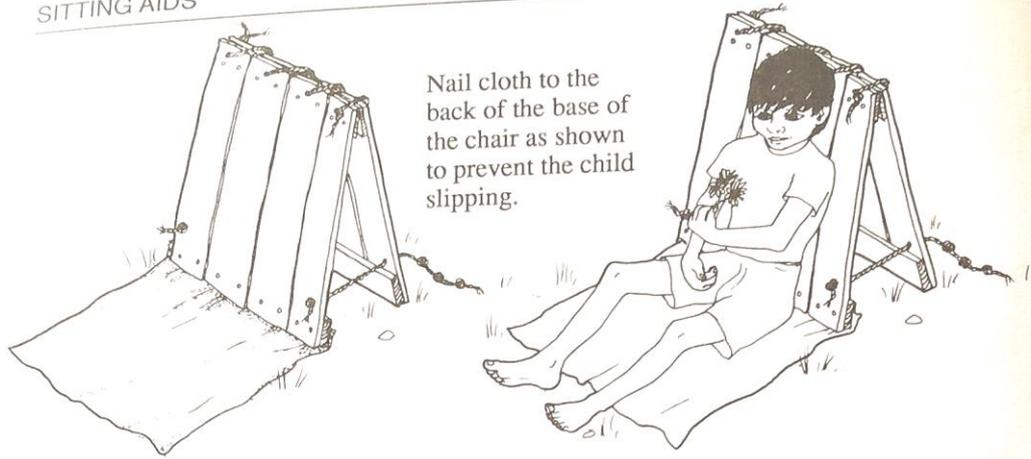
Nail cloth to the back of the base of the chair as shown to prevent the child slipping.
