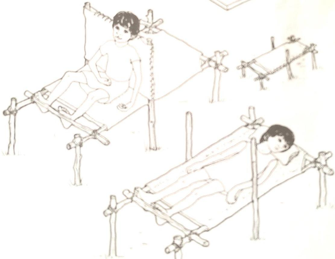
4. A removable back support means that a chair can be converted into a bed.
